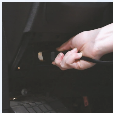
Plug in the connector to the vehicle's OBDII port
