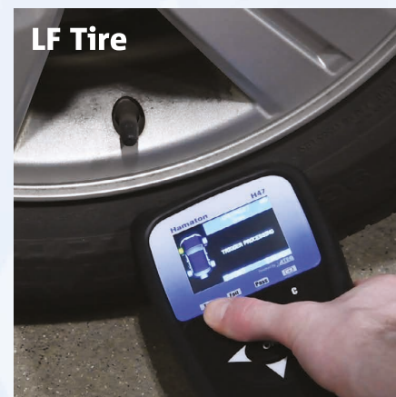
Place the tool on the sidewall near the valve, then press the green trigger button
