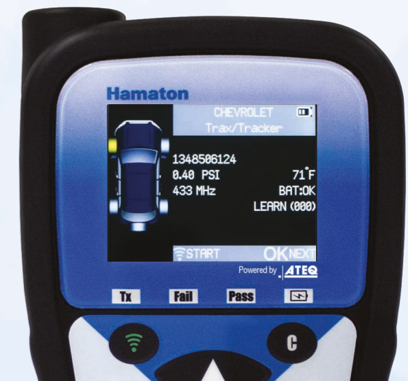
The tool will display the sensor's ID, battery status and frequency besides the tire's pressure and temperature
